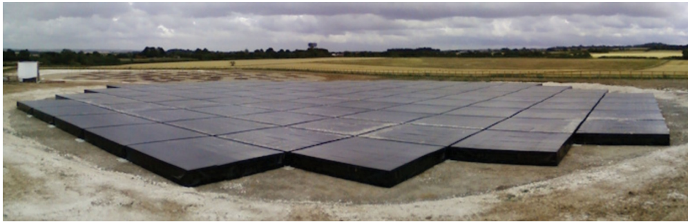
Figure 4. The Low Frequency Array (LOFAR) is an industrially produced multi-purpose sensor array concept for mainly radio astronomy at low frequencies below 250 MHz. Several sites have been constructed across Europe, the latest one being the LOFAR-UK Chilbolton site. The image shows the so-called High-Band Array (HBA) 120-250 MHz. The antenna array consists of 96 element tiles, having altogether 3072 individual antenna elements. The HBA can be used as a receiver for the EISCAT_3D and the existing EISCAT VHF radars. During the Preparatory phase action, University of Oulu will install one LOFAR remote site with 48 HBA tiles at Kilpisjärvi in Finland. Prototyping of the EISCAT_3D beamforming will be tested in bi-static measurements using the current EISCAT VHF transmitter from autumn 2011.
