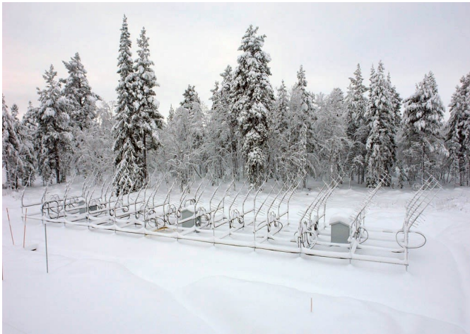
Figure 2. A small 224-MHz receive-only antenna array was constructed during the EISCAT_3D Design Study 2005-2009 at the Kiruna EISCAT site. The demonstrator array is a rectangular, 12x4 array of (6+6) element X-Yagis, with its major axis aligned in the Kiruna-Tromsø plane. Antennas operating in an Arctic environment will have their performance degraded significantly due to snow and hoarfrost sticking to the antennas. This aspect was among the topics investigated during the Design Study.
