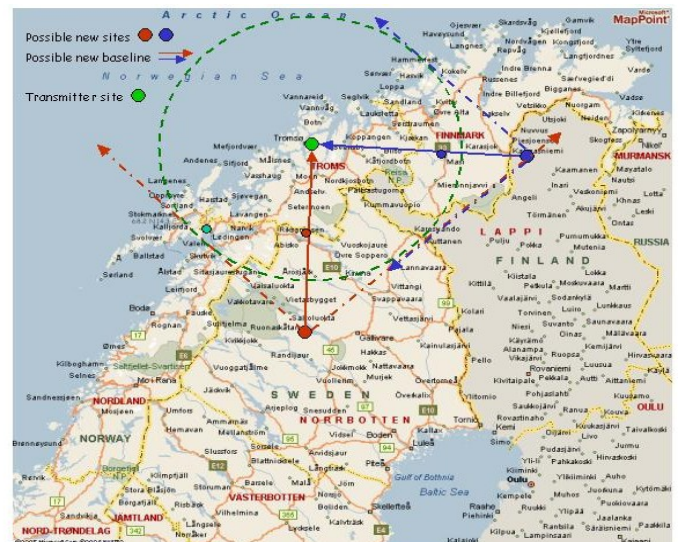
Figure 3. Geographical layout of the transmitter and receiver sites, as proposed in the EISCAT_3D Design Study 2005-2009. The dashed circle indicates the approximate extent of the common field-of-view at 300 km altitude. Options for locating the active and passive sites will be re-investigated during the Preparatory Phase action in 2010-2014. Several active sites are envisaged in the final configuration of the EISCAT_3D radar.
