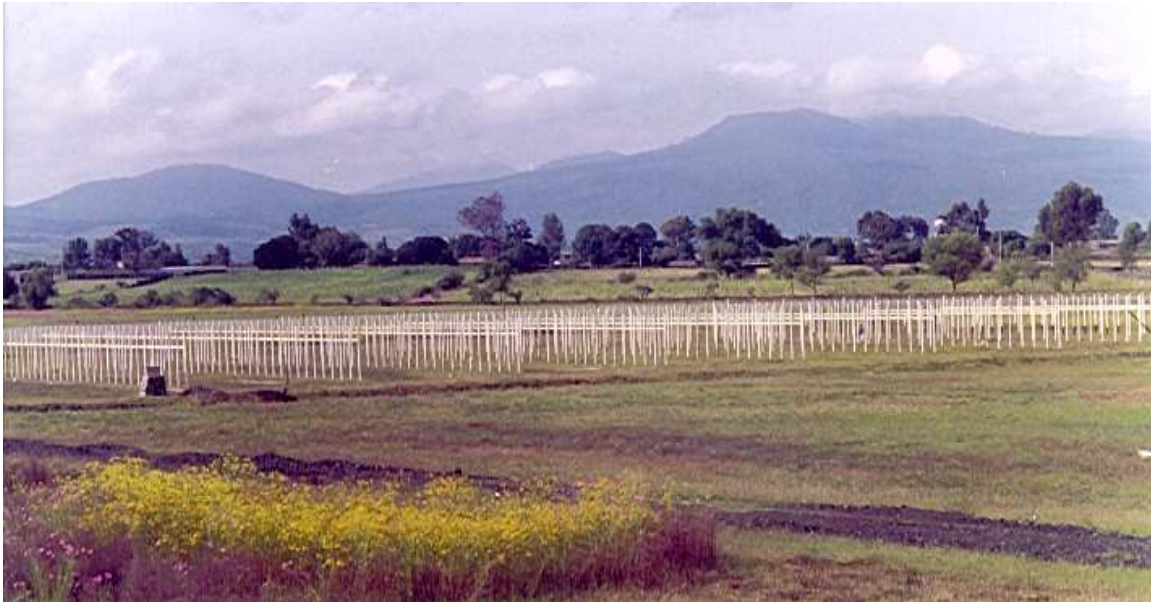
Figure 3. The MEXART 10,000 m 2 , 140 MHz, radio array located in Michoacán, México (see website: http://www.youtube.com/watch?v=GNadikiR-IQ ).
